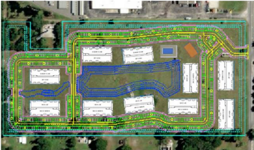
Example of concept plan prepared in OpenSite™
