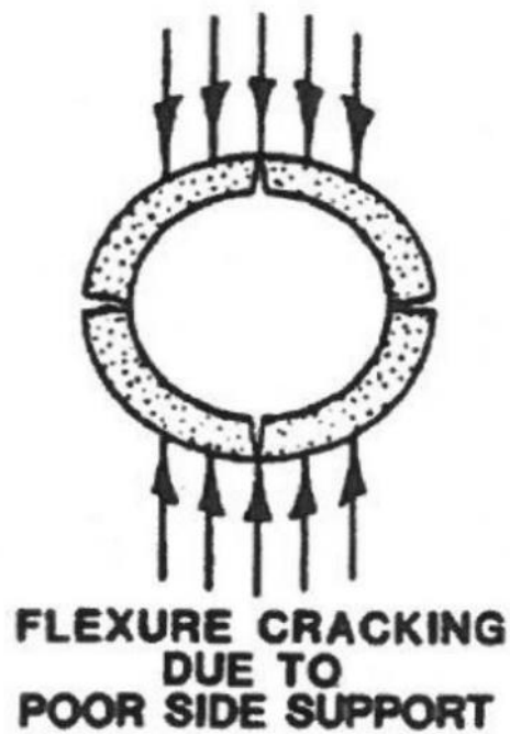
Figure 4.10.2-1—Results of Poor and Good Side Support in Rigid Pipe
