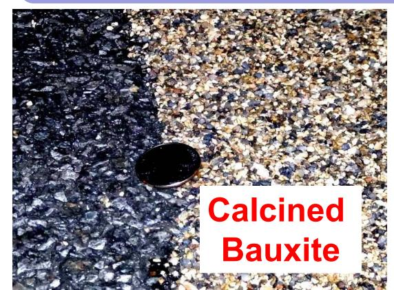
3 mm aggregate pavement surfacing overlay systems used for spot Safety Treatments
